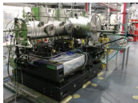
Three interchangeable gratings installed in the BOREAS monochromator at ALBA synchrotron
