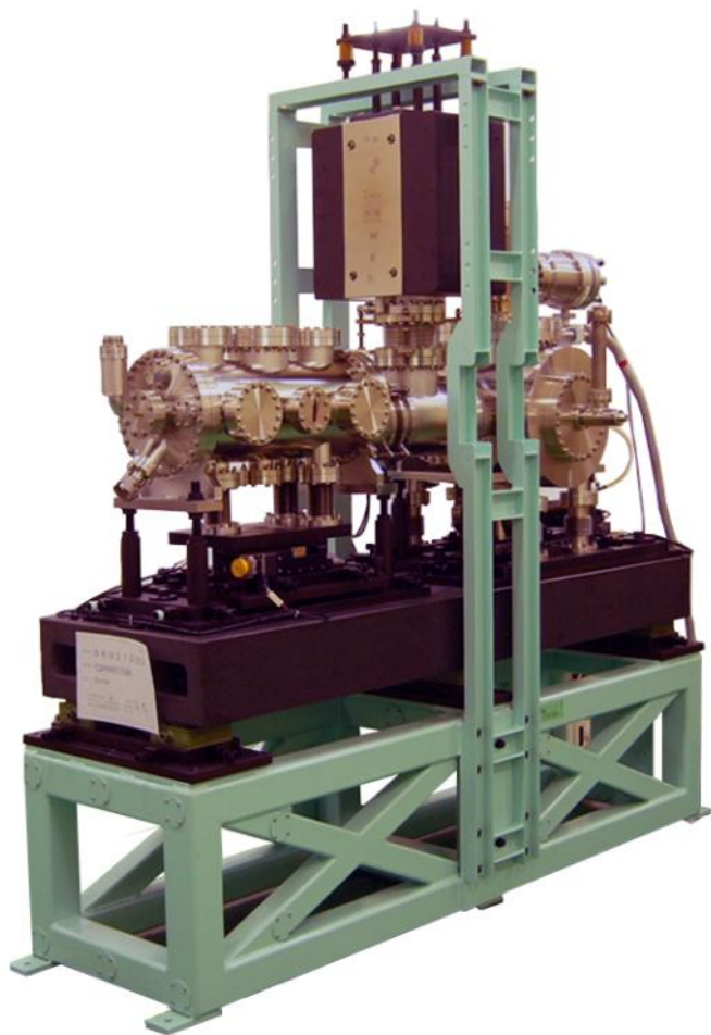
VLSPGM monochromator installed on the Metrology and Tests beamline at the SOLEIL synchrotron
