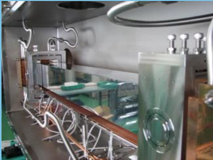
Liquid nitrogen cooled mirror system
