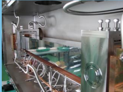
Liquid nitrogen cooled mirror system
